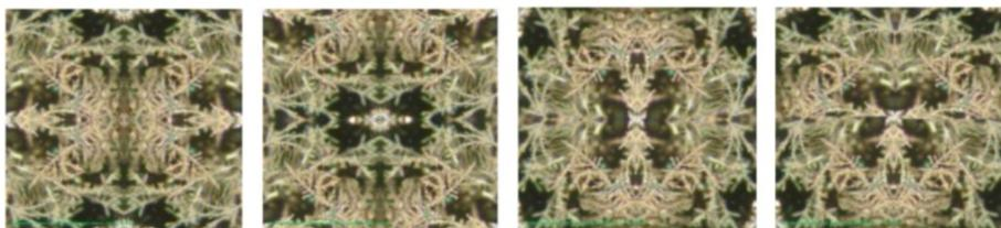
**Figure 2.** Growth of dendritic lead crystals from the reaction of zinc with lead nitrate 0.1 M solution.
